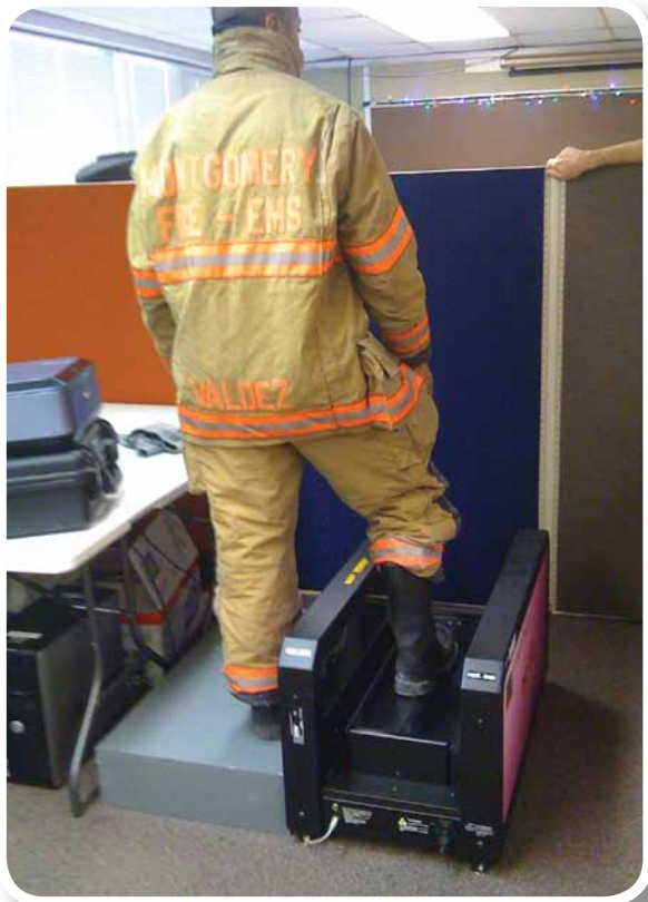
Firefighter having boot scanned in foot measuring unit.
