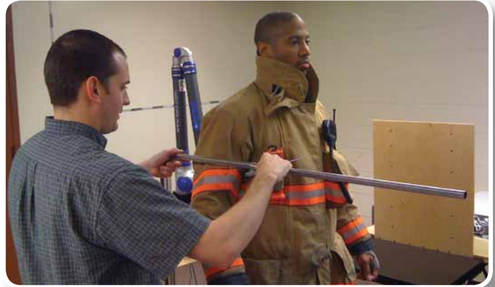
Physical measurements are taken of each subject in order to compare results with the laser scan.
