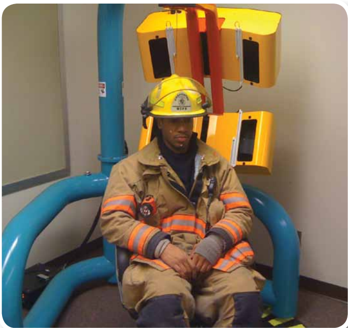
Full body scan of firefighter in seated position with turnout gear.
