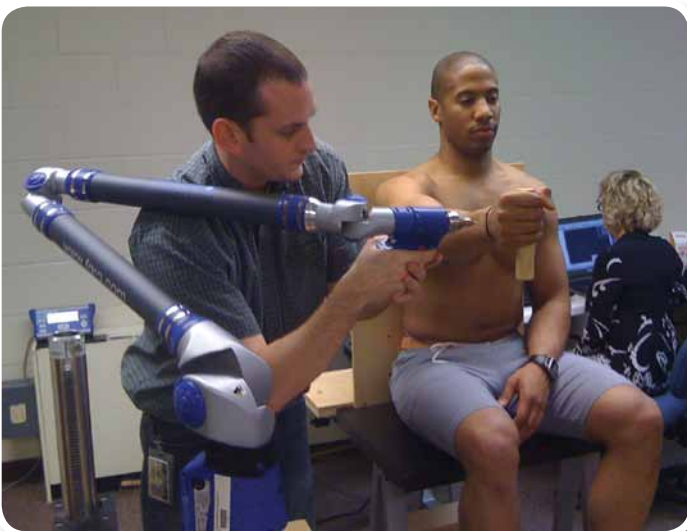
Staff uses electronic measuring device to pinpoint specific measuring points on the firefighter’s body.
